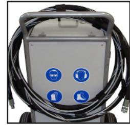
Integrated holding device for hose
