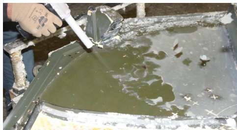
Cleaning of a mould in PU-production
