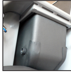
Insulated pellet hopper with 6kg (13.22lb) capacity
